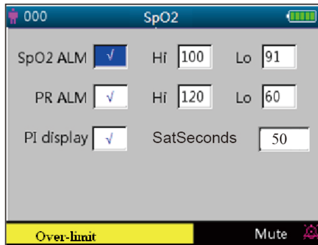
Figure 4.12C SpO 2 Setup Screen (with Nellcor SpO 2 configuration)
